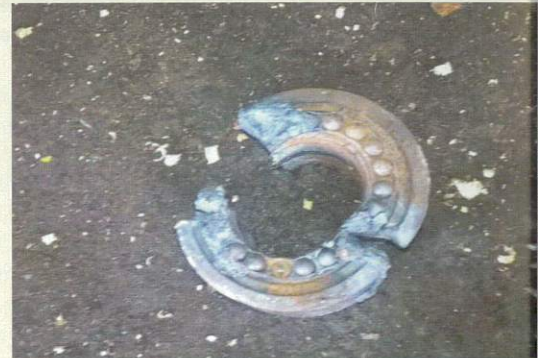
Thrust bearing found damaged
